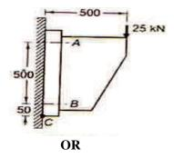
5a) What is an eccentric riveted joint? Explain the method adopted for designing such a joint?
